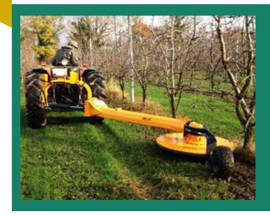
Mechanical driven swing arm mower can be used to mow around trees, posts, crash barrier, etc. Without any damage.
