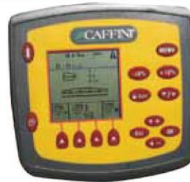
**Computer "Compact"** for the automatic control of the treatment. The display shows l/ha during the treatment, the sprayed litres, the treated area.
