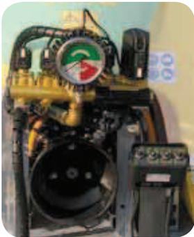
**Electric distributor "Plus"** complete with 2 motorized compensated valves, electric valve for pressure adjustment and general electric closing. Self-cleaning filter and manometer Ø 100 mm complete the equipment.
