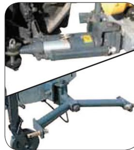
**Steering draw bar with central attachment** or with 3 point attachment.
