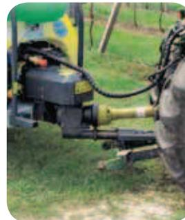
**Steering draw bar with gear** (offered from Caffini since 1982) allows narrow steering angles and the PTO shaft joints always in line.
