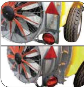
**Rear lights:** folding system. "Open" during use on street could be "closed" during work in field.
