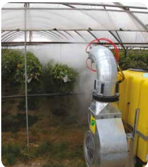
The "Turbine Overland" mist-blower has been realized for middle-high cultivations in open fields or out of fields in greenhouses. The cannon head could rotate 180° on horizontal line, thanks to the hydraulic motor A (optional) or manually. "Overland" is provided with a smart high adjustment B to be adapted to the different height of treatment.
