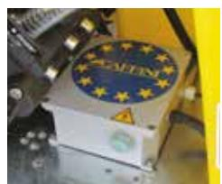
Thanks to the electrostatic charge the chemical droplets are attracted by the vegetation leaves-branches, reducing the drift.
