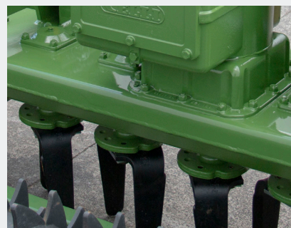
Fully welded gearbed
