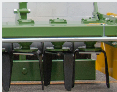
Wide spaced bearings on rotors
