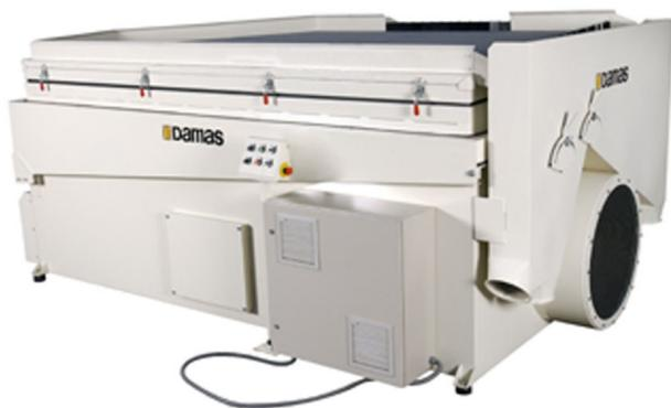
Zeta gravity separators are used to separate products with difference in specific weight.
