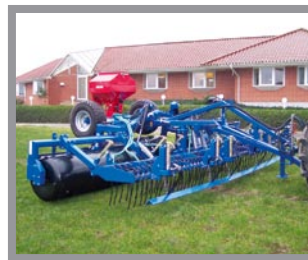
Lower the side sections and lift the wheels
