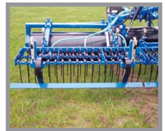
Set torsion to side sections hydr. valve in float position.
