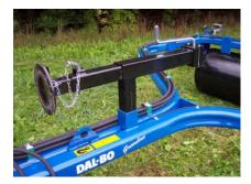
During transport the support leg is placed in a special bracket.
