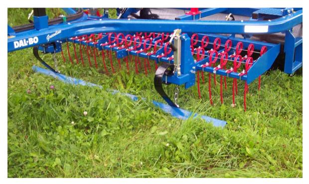
The 2 row weed harrow, which is hydraulic adjustable, aerates the grass with 12 mm spring tines. To level mole hills and other irregularities the **Greenline 300** can be fitted with, as the name indicates, a mole hill board in front of the harrow. The depth is adjusted by spindles.
