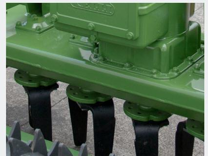
Fully welded gearbed
