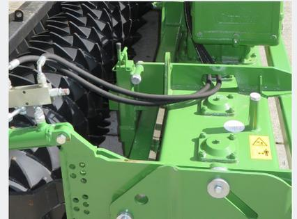
Leveling bar attached to gearbed
