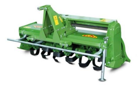
An important feature of side shift rotary tillers is that they till soil both from the center and the sides with respect to the centerline of the tractor. This allows operation in areas that the tractor cannot reach due to its height (for example, under trees or near greenhouse walls). The gearbox always remains in the center so that the drive shaft always operates in a straight position, while the whole machine body shifts sideways.
