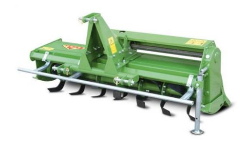
An important feature of side shift rotary tillers is that they till soil both from the center and the sides with respect to the centerline of the tractor. This allows operation in areas that the tractor cannot reach due to its height (for example, under trees or near greenhouse walls). The gearbox always remains in the center so that the drive shaft always operates in a straight position, while the whole machine body shifts sideways.
