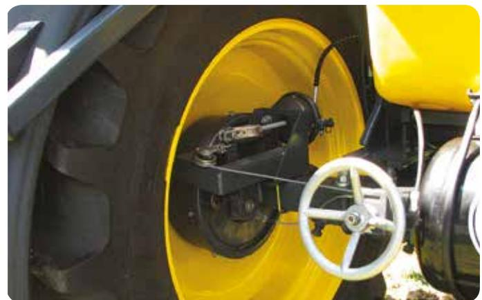
**Brakes:** these are available in hydraulic or pneumatic, with manual control or automatic with the tractor pedal. Road regulations of 25km/h or 40 km/h or 50 km/h (Germany).
