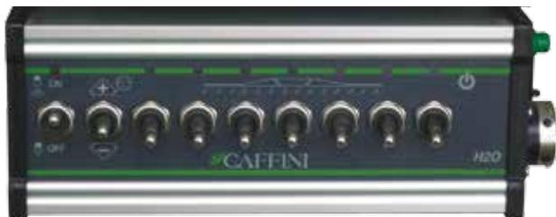
**"Electrocontrol"**: a block of 5/7/9 electric motor valves for the section of the boom. This block also has an electric valve for general closing (by pass) and electric adjustment of the pressure. The functionality of the electric distributor is guaranteed from a practical self-cleaning filter.
