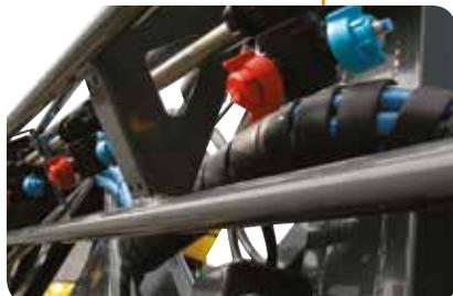
The nozzles and tips are protected inside the boom structure in order to avoid any contact with the ground or obstacles. The pipes are in stainless steel. The optional "trijet, quadrijet or pentajet" nozzles are fitted with anti-dripping membrane device, shutdown position and the ring nuts are of the "quick coupling type".
