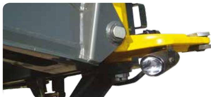
**Set night-work lights:** positioned in the centre of the bar, these special long beam lights enable visibility of the nozzles during night-time treatments.
