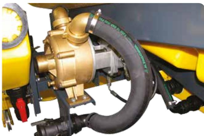
**Centrifugal pump:** these are available as optional for loading activated by hydraulic motor with flow rates of 250 and 500 l/min.
