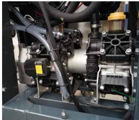
**The two high-flow pumps** connected in tandem are made with anti-corrosive raw materials. One pump is for the treatments and the other one is for the recovery of the drops catch from the panels.
