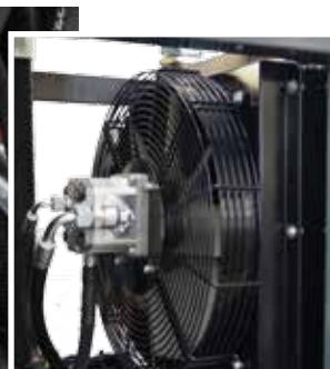
**Independent hydraulic system** made with high-quality components: this system powered by the tractor PTO, includes a large oil tank and oil cooler.
