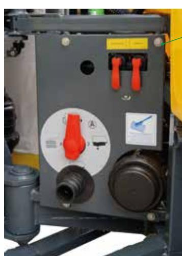
**"Hub Service"**: work station at left side of the machine for preparation of spraying treatments. The valves functions are guided by coloured pictograms. Comfort and time saving!
